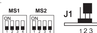
position of MS1 , MS2 microswitches and jumper J1 to exit the programming phase.
